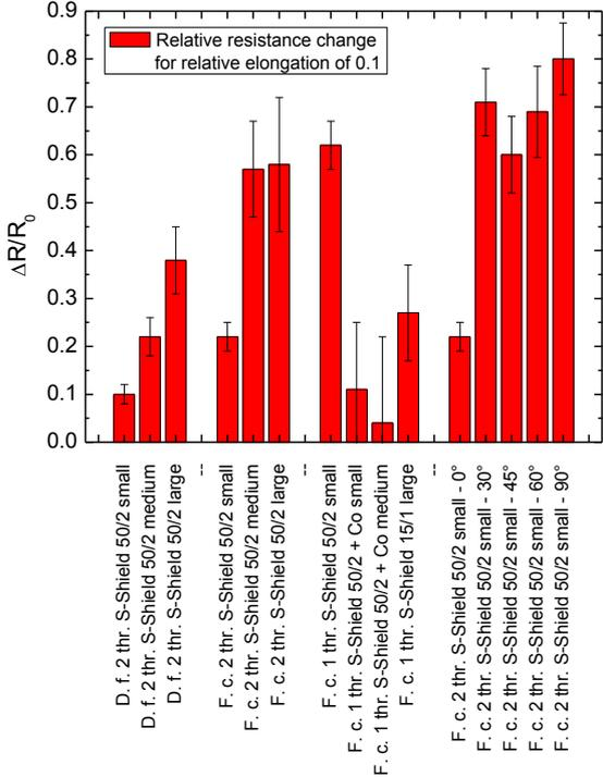
Fig. 7: Comparison of different structures knitted from various yarns, as described before. D. f. = double face, F. c. = full cardigan, thr. = threads. The relative resistance change  $\Delta R/R_0$  is defined as  $1 - R/R_0$  and has been detected here for a relative elongation of 0.1. The error bars
